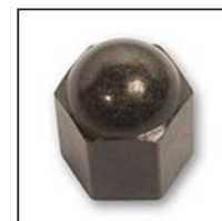
Acorn Nut P/N 81600189 Tighten to 20 ft/LBS.
