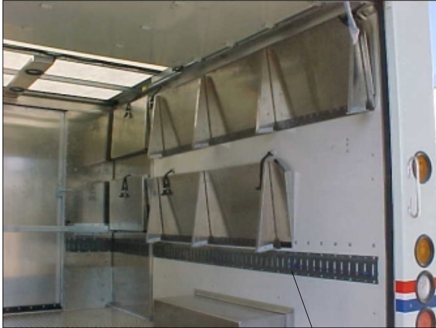
001739501 Track Retainer x 32.00" (2 ea.) 001739502 Track Retainer Left x 26.00" (1 ea.) 001739503 Track Retainer Right x 18.00" (1 ea.)
