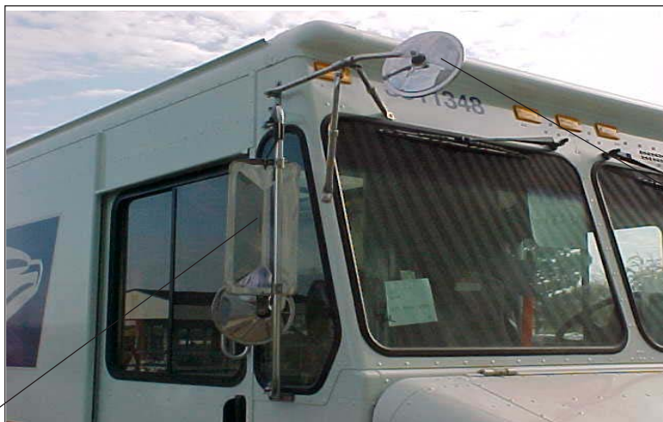
47005097 Mirror Crossview Front (1 ea.) 47005100 Mirror Bracket Kit Front (1 ea.) 47005101 Mirror Head 8" (1 ea.)
