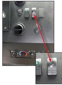
A door lock switch is located on the dash panel. Pressing the switch once will unlock both the passenger and driver side doors. *Note: The doors will relock if not opened within six seconds.*
