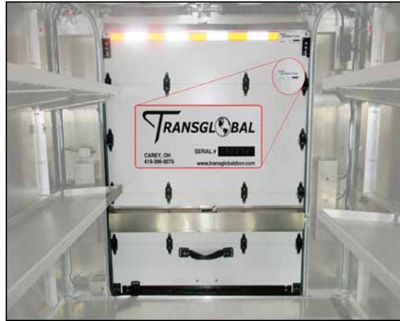
ROLL-UP DOOR SERIAL NUMBER LOCATION
