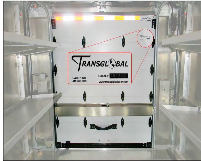
ROLL-UP DOOR SERIAL NUMBER LOCATION
